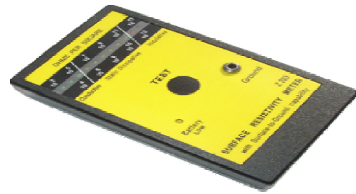
Surface Resistivity Meter
